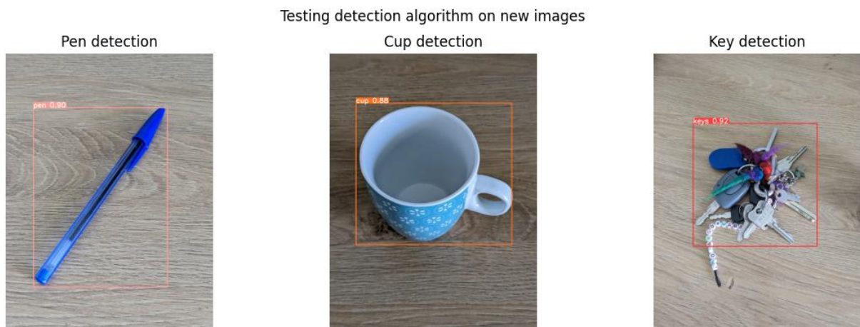
Fig. 2. Predictions on images from outside the dataset, the confidence of the object detections were pen 0.9, cup 0.88 and keys 0.92.
