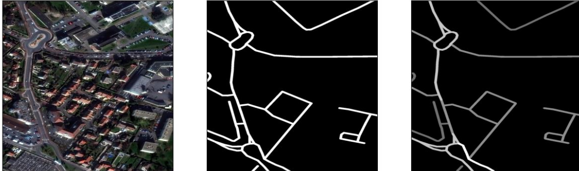
Figure 3. Left: sample training image in Vegas. Middle: typical binary training mask. Right: continuous mask where the mask value is proportional to the value of interest (in this case, speed limit).
