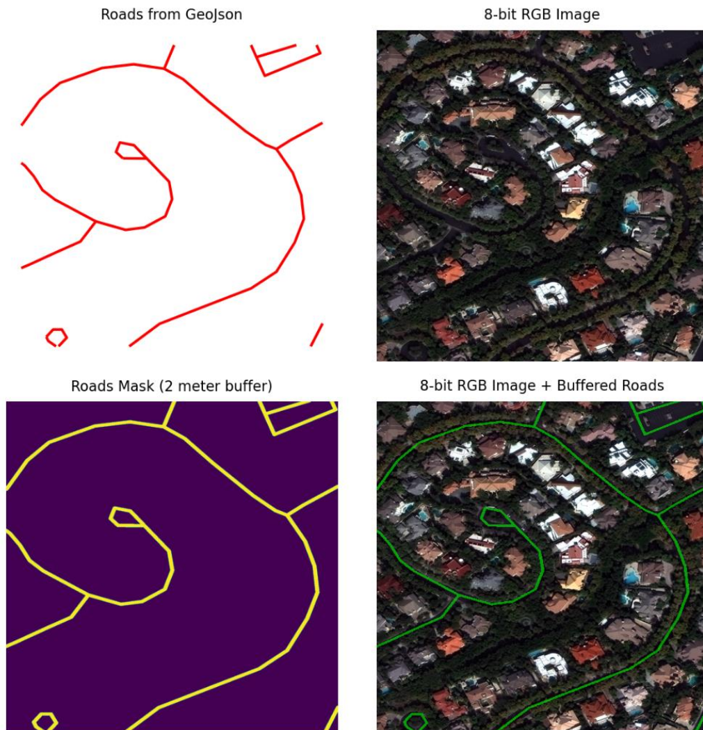
Figure 1. An example of the segmentation mask generating script's output. The raw GeoJSON label is shown in the top left, while the equivalent 8-bit RGB picture is shown in the upper right. The lower-left illustrates the output of the script: the pixel mask inferred from the GeoJSON label. The road mask is overlaid over the RGB picture in the lower right.
